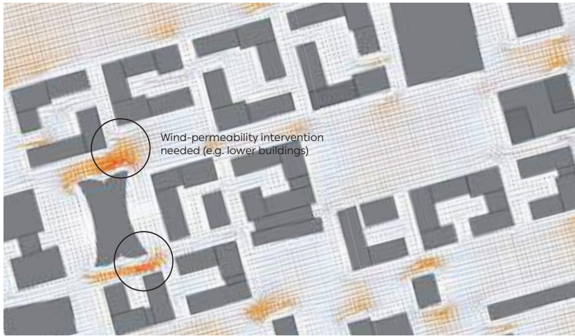
▲ Computational Fluid Dynamics (CFD) Simulation of Vaso Miskin Crni representing the wind conditions in Sarajevo, Source: ETH Zurich, Prof. Hubert Klumpner and Dr. Michael Walczak
